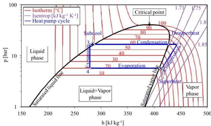
Figure 2.6 Log p,h diagram of a theoretical vapor compression heat pump cycle; Working fluid R134a;  $T_{\text{cond}} = 60\text{ }^{\circ}\text{C}$ ;  $T_{\text{evap}} = 20\text{ }^{\circ}\text{C}$ ;  $\eta_s = 0.8$ ; Superheat = 5 K; Subcool = 5 K; Isenthalpic expansion
