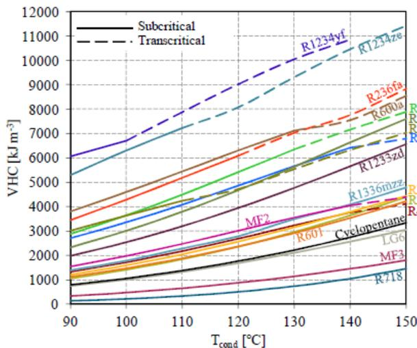
Figure 3.12 VHC of all considered working fluids over the temperature range  $T_{\text{cond}} = 90 - 150$  °C; Superheat = 5 K; Subcool = 5 K;  $T_{\text{th}} = 50$  K;  $T_{\text{increment}} = 10$  K;  $\eta_v = 0.8$ ; Isenthalpic expansion;  $\Delta T_{\text{HX}} = 5$  K; No IHX for R718
