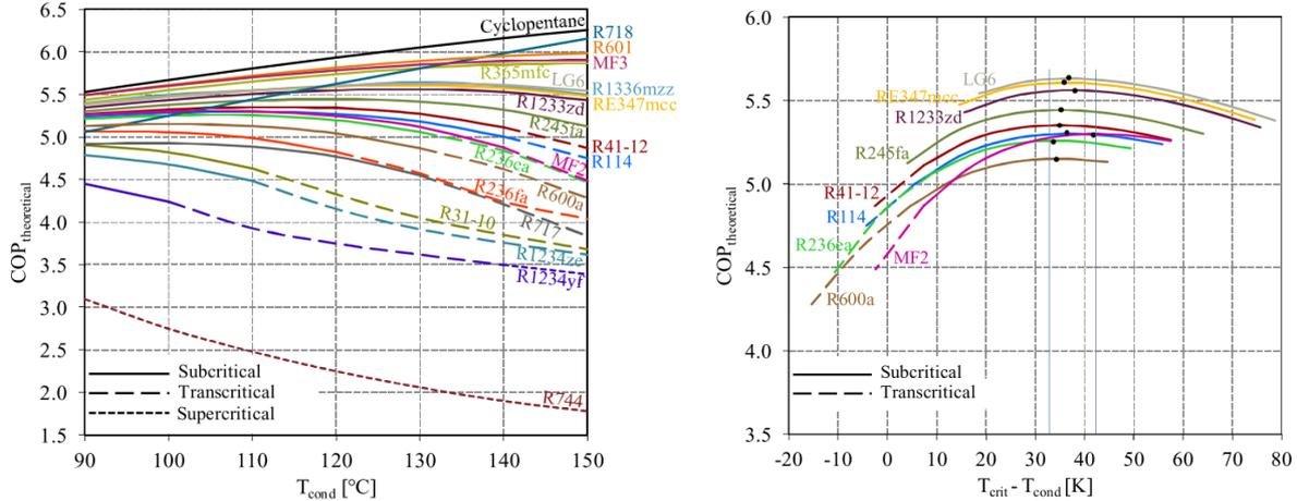
Figure 3.7 Theoretical COP of all considered working fluids over the temperature range  $T_{\text{cond}} = 90 - 150$  °C; Superheat = 5 K; Subcool = 5 K;  $T_{\text{th}} = 50$  K;  $T_{\text{increment}} = 10$  K;  $\eta_v = 0.8$ ; Isenthalpic expansion;  $\Delta T_{\text{HX}} = 5$  K; No IHX for R718, R717
