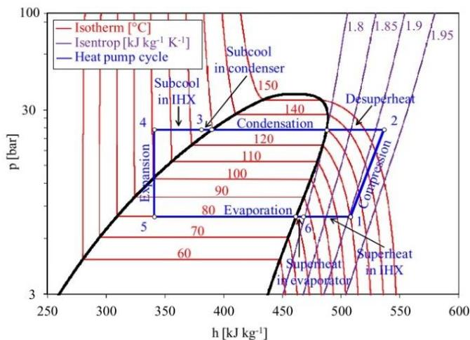
Figure 3.4 Log p,h diagram of a theoretical vapor compression heat pump cycle with IHX at subcool case 1 (cycle type 1); Working fluid R245fa; Standard simulation point  $T_{\text{cond}} = 130\text{ }^{\circ}\text{C}$ ;  $T_{\text{evap}} = 80\text{ }^{\circ}\text{C}$ ;  $\eta_s = 0.8$ ; Superheat = 5 K; Subcool = 5 K; Isenthalpic expansion;  $\Delta T_{\text{IHX}} = 5\text{ K}$
